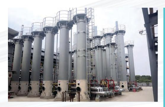
Hydrogen can be recovered by the pressure swing system from very different feed gases, e.g.:
